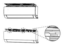
3. Push down hooks to assemble the air filter.
