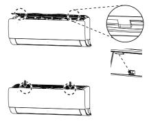
4. Check side of the front grille for the air filter assembled correctly.
