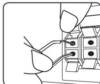
Connect the black stripe of each wire to the terminals marked -(minus) and the other end to the terminals marked +(plus).
