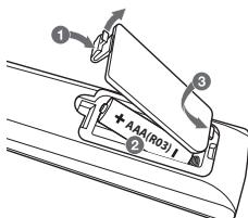
Remove the battery cover on the rear of the Remote Control, and insert R03 (size AAA) battery with  $+$  and  $-$  matched correctly.
