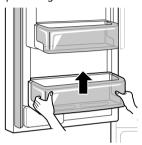
**2** To assemble the baskets, slide it in above the desired support and push down until it snaps into place.
