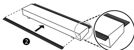
7 Attach the lower cover with the strip onto the appliance.
