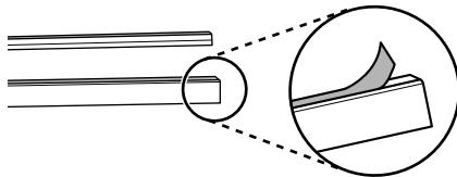
5 Attach the black coloured lower strip ① to the bottom of the lower cover.
