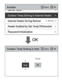
Set whether to use the "Outdoor Temp Setting in Internal Heater" function and the outdoor temperature value.
