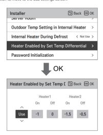
Set whether to use the "Heater Enabled by Set Temp Differential" function and the heater operation temperature difference value.
