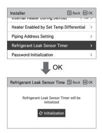
Please make sure to reset the refrigerant leakage detection sensor, if you replaced it.
