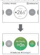
In case of air purify single operation, it operates in fan mode / automatic wind state, and the wind direction operated before the air purify single operation is turned off.
