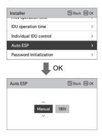
After selecting the voltage setting, the product will automatically operate and automatically set the rotation speed for each fan speed - High, Medium, and Low.
