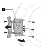
3 Remove the 3 screws from the door latch assembly which is fixed between the door and the hinge assembly, and then remove the screw which is fixed on the door hook.
