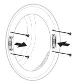
7 Install the door with the screws removed in step 1 and then check the door closes properly.
