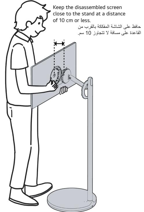
**7** Press the plug lock, push it in the direction of the arrow, and then disassemble the screen completely.
