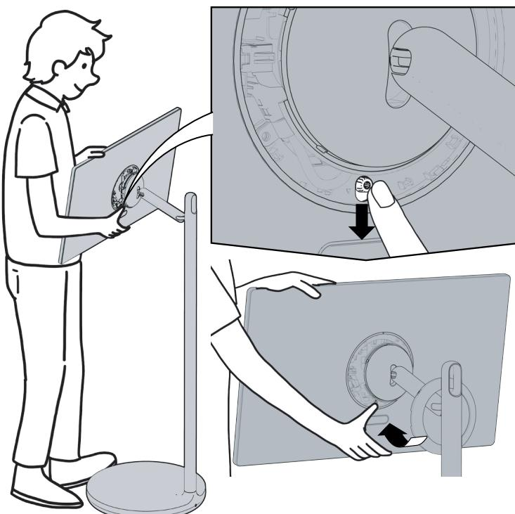
**6** Lift the screen, separate the top of the screen, and hold the screen.
