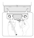
3. Remove the Wall bracket install guide.
