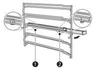
2 Rotate the telescopic runners anti-clockwise (clockwise for right side) by 90 degrees.
