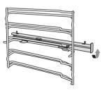
3 Push forward the telescopic runners, make the side rack buckled onto the lower wire and
