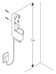
5 Attach the charging station to the wall with the wall anchoring screws.
