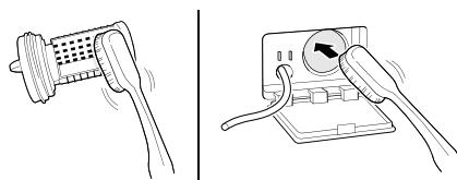
**6** After cleaning the drain pump filter, carefully reinser the filter and screw the drain cap back in clockwise carefully to avoid cross threading and leakage.
