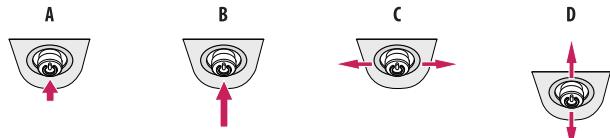
**A (Power on):** Press the joystick button once with your finger to turn on the monitor.
