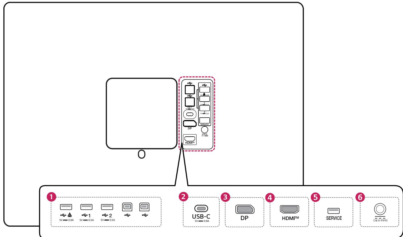
**1 USB IN 5 V — 0.5 A, USB IN (A) 5 V — 0.9 A, USB UP**
