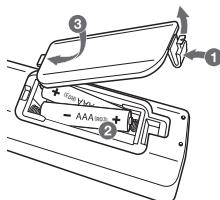
Remove the battery cover on the rear of the remote control, and insert the battery with **+** and **-** matched correctly.
