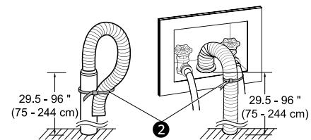
**Using a Standpipe to Drain**
