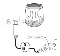
If the battery is fully charged in charging mode, **EED** (RED) is turned off.
