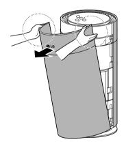
2 Using a vacuum cleaner or soft brush, remove any dust from the pre-filter surrounding the filter.
