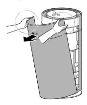
3 Remove the filter and detach the vinyl.
