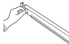
**2** Fit the side bracket to the side of the washer top as shown. Firmly press the adhesive area of the bracket to the washer surface. Secure the side bracket to the washer with a screw on the back side of the bracket. Repeat steps 1 and 2 to attach the other side bracket.
