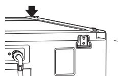
**3** Place the appliance on top of the washer, fitting the dryer feet into the side brackets as illustrated. Avoid finger injuries; do not allow fingers to be pinched between the washer and
