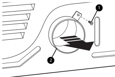
**2** Press the adapter duct **3** onto the blower housing and secure it to the base of the appliance as shown.
