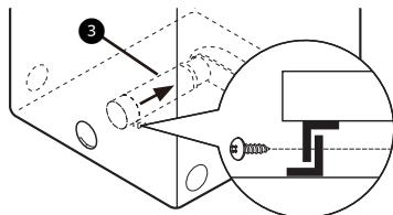
**3** Insert the 10.2 cm elbow **4** through the rear opening and press it onto the adapter duct. Be sure that the male end of the elbow faces down through the hole in the bottom of the appliance. Secure it in place with duct tape. Attach the cover plate **5** to the back of the appliance with the included screw.
