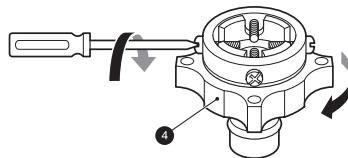
2 Remove the guide plate ⑤ if the tap is too large to fit the adapter.
