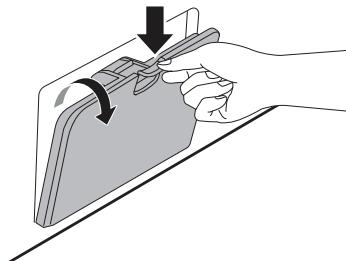
**3** Remove the drain plug from the drain tube first, and then drain the water.
