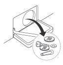
4 After cleaning, turn the pump filter and insert the drain plug.
