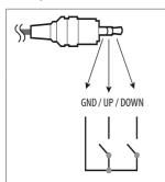
Each up/down pins are connected to CPU with pull up resistor respectively.
