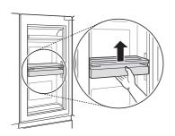
To lower the moving basket, press up to release the levers at the side of the basket and lower the basket until it clicks into place.
