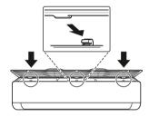
**6** To make sure the filter is assembled properly, press down along the entire front length of the filter.
