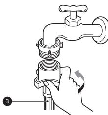
connector latch plate. Make sure the adapter locks into place.
