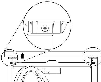
2 Pull the top cover backwards after removing the two screws and then lift it up to remove it.
