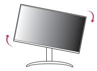
4 Complete the installation by rotating the monitor 90° as shown in the figure.
