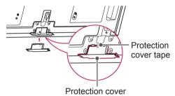
3 Assemble the parts of the Stand Pole with the
