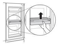
2 To lower the moving basket, press up to release the levers at the side of the basket and lower the basket until it clicks into place.
