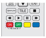
2 To change the Picture ID, press the ON button, or the left and right arrow buttons continuously. Assign the ID you want.
