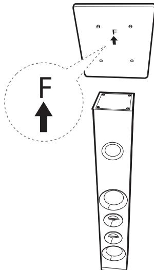
3. Tighten up with supplied screws.
