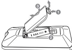
Remove the battery cover on the rear of the remote control, and insert the battery with  $\oplus$  and  $\ominus$  matched correctly.
