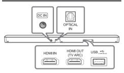
Make sure to properly align and connect the optical cable; improper alignment may cause damage to the jack.
