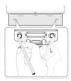
3. Remove the Wall bracket install guide.
