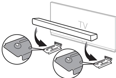
8 Firmly attach the product to the wall brackets using the screws provided.
