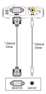
You can connect the audio cable without using a gender as shown in the illustration above.
