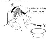
3 Remove any extraneous matter from the pump filter.
