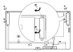
3 Then connect the speaker cable. After installing your speakers, use holders and cable ties to organize the speaker cables.
