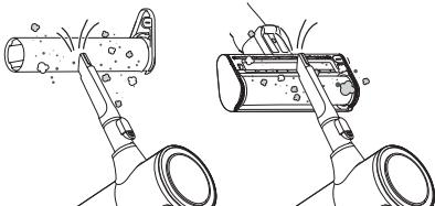
5 Use a damp towel or cloth to remove any remaining foreign objects and dust from the brush and the bottom of the nozzle. Remove foreign objects, debris and hair from all Rollers of the nozzles using tweezers.
