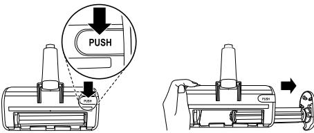
**3** Attach the crevice tool to the product body and use the vacuum to remove foreign objects and dust from the brush and the bottom of the nozzle.
