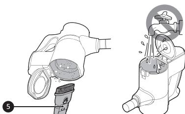
**7** Turn the product body over and lift the Kompressor lever ⑥ up to clean the inside of the working plate with the cleaning brush, etc.
