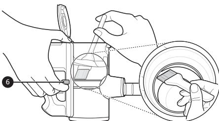
**8** Turn the product body over again and shake it while pressing down the lever to remove the dust.
