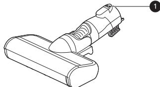
2 Turn the nozzle upside down and remove the rotating brush while holding down the **PUSH** button on the nozzle.
