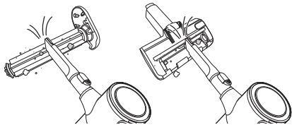
**4** Use a damp towel or cloth to remove any remaining foreign objects and dust from the brush and the bottom of the nozzle. Remove foreign objects, debris and hair from all Rollers of the nozzles using tweezers.
