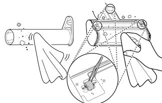
2 Turn the nozzle upside down and rotate the cover lock slot ② counterclockwise.
