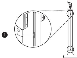
3 Slide the detachable nozzle storage onto the floor stand pipe.
