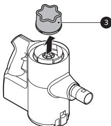
6 Insert the dried pre-filter and rotate the exhaust filter to the locked position ⑤ to reassemble it on the product body.
