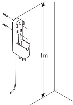
**3** Attach the charging station to the wall with the wall anchoring screws.
