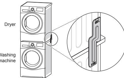
This dryer may only be stacked on top of an LG washing machine. Do not attempt to stack this dryer on any other washing machine, as damage, injury or property damage could result.
