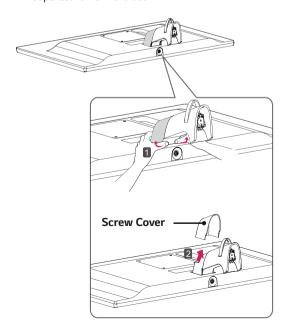
4 Remove the two screws on the back of **stand body**.
