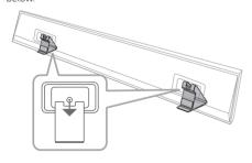
When installing the sound bar with a stand, install it so that it does not cover the TV's remote sensor or screen.
