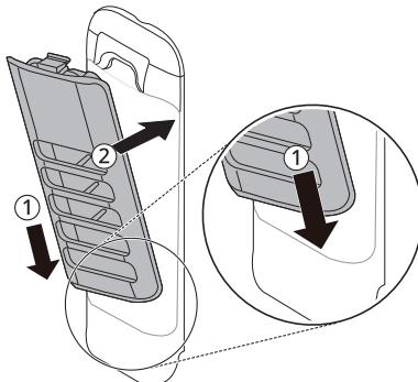
1 Push down on the release tab on the top of the filter cover and pull forward.
