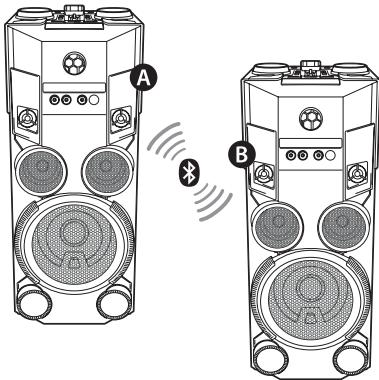
1. Press and hold **F / WIRELESS LINK** on the unit for 3 seconds. PARTY LINK MODE SELECT appears in the display window.
