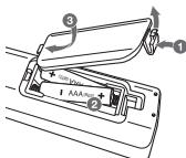
Remove the battery cover on the rear of the remote control, and insert the battery with **+** and **-** matched correctly.
