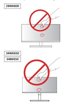
If you use the monitor panel without the stand base, its joystick button may cause the monitor to become unstable and fall, resulting in damage to the monitor or human injury. In addition, this may cause the joystick button to malfunction.
