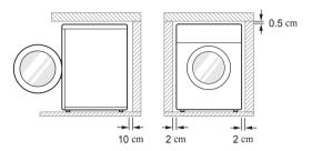
**Level floor**: Allowable slope under the entire washing machine is 1°.
