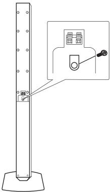
Connect the speaker wire to the terminal on the speaker. Make sure the wire marked black goes in to the terminal marked "-"(minus) and the other wire goes in to the terminal marked "+"(plus)
