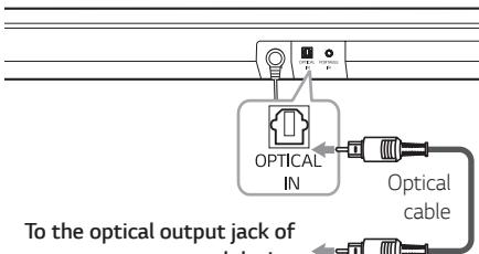
1. Connect the OPTICAL IN jack on the back of the unit to optical out jack of your external device.
