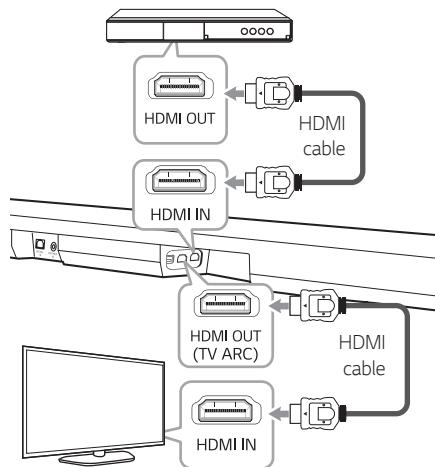
1. Connect HDMI IN jack on the back of the unit to HDMI OUT jack on the external device such as Blu-ray disc player, DVD player, etc.
