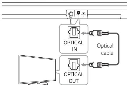
2. Select the input source to OPT/HDMI ARC by pressing **F** button on the remote control or unit repeatedly.
