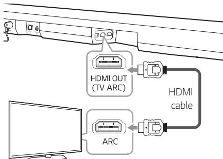
2. Select the input source to OPT/HDMI ARC by pressing **F** button on the remote control or unit repeatedly.
