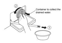
3 Remove any extraneous matter from the pump filter.
