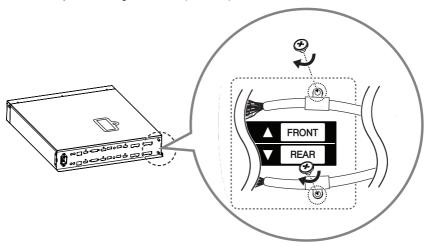
4 If installing onto a ceiling or wall, attach the mounting brackets to the Signage box using four screws (M4 x L8).
