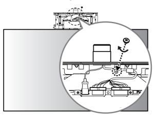
11 When installing the product to a stand (excluding a ceiling mount or a wall mount), remove the 2 screws, change the direction of the LG logo, and then reassemble it.
