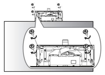
13 Cover the REAR side with the other T-con box cover and attach it using 2 screws ( $\Phi$ 3 x L10).
