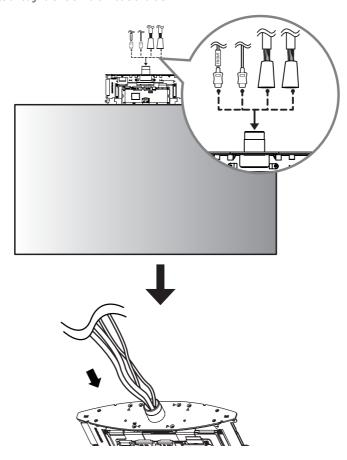
9 Connect the HDMI cable with the label marked 'FRONT' to the FRONT side. Insert the 16/22 pin cable with the red mark to the cable holder and connect it using a screw (M3 x L4.5).
