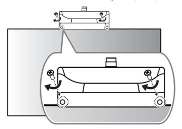
14 Attach the bottom part of the T-con cover using 6 screws (M4  $\times$  L10).
