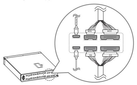
3 Attach the 16/22 pin cables using the 2 screws (M3 x L4.5).
