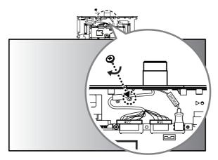
10 Connect the HDMI cable (without the label marked 'FRONT') to the REAR side. Insert the 16/22 pin cable (without the red mark) to the cable holder and connect it using a screw (M3 x L4.5).
