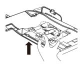
2. Open the front panel and lower the PM1.0 Sensor case as shown in the figure below.
