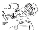
3. Once the PM1.0 Sensor case is lowered all the way, turn the PM1.0 Sensor case to secure it as shown in the figure below.
