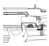
4. Open the PM1.0 sensor cover on the side of the case.
