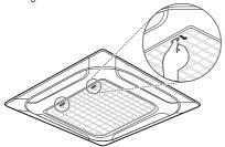
2. Remove PM1.0 filter by pressing the fixing hook.
