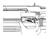
5. Use a slightly wet cotton swab to wipe dust off the lens, and then use a dry swab to remove the moisture.
