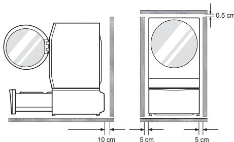
**Level floor** : Allowable slope under the entire appliance is 1°.
