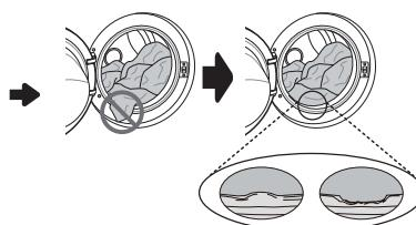
Leakage caused by the damaged gasket. The gasket is damaged because the clothes are jammed between the door glass and the gasket.
