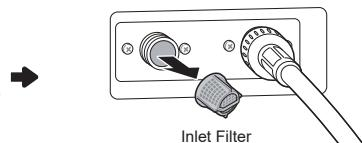
Clean the inlet valve filter or reinstall the water supply hoses.
