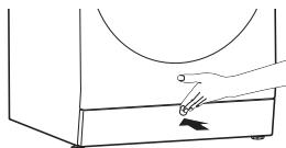
2 Unplug the drain plug and open the filter by turning it to the left.
