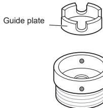
3 Push the adapter onto the end of the tap so that the rubber seal forms a watertight connection. Tighten the four fixing screws.
