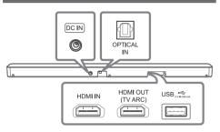
If the optical cable is not connected in the correct direction, it may cause damage of optical jack.
